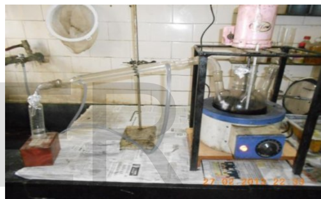
Fig. 4 Batch Process For Transesterification
